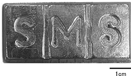
Fig. 5 Zinc ingot from seafloor massive sulfides
