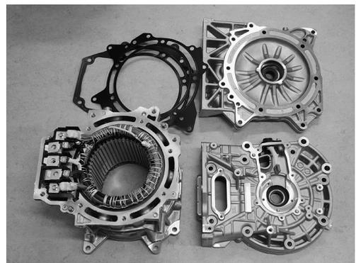
Fig. 1 Housings and stator for the drive motor of an electric vehicle.
